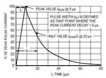
Figure 3.  $8 \times 20~\mu s$  Pulse Waveform
