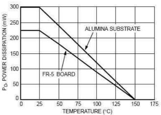
Figure 2. Steady State Power Derating Curve
